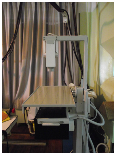
Fig. 1. Photo of digital X-ray diagnostic complex KRDTs-o8-ALPHA with the position of the table for radiography with magnification mode
