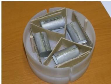
Figure 2 Two layers of TLD dosimeters in cadmium cylinders and polyethylene box.
