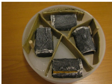
Figure 3 Two layers of activation foils in boron carbide cylinders and PE box.
