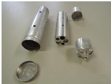
Fig. 3 A capsule with samples is in the middle, a standard capsule used in the reactor is on the left, the lid with the experiment number is in the foreground
