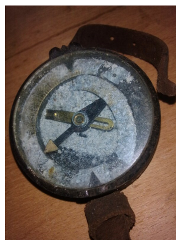
Picture 2 Compass with decomposed radium paint
