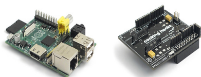
Fig. 7 Radiation Sensor Board for Arduino / Raspberry Pi pack and Raspberry Pi to Arduino Shield Connection Bridge
