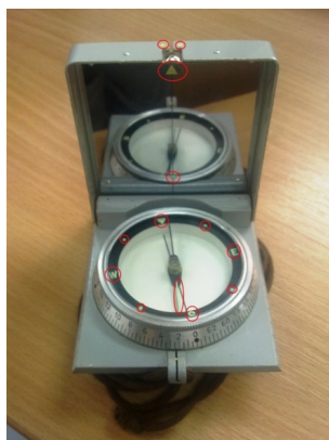
Picture 1 Ra-226 and tritium paint on compass body
