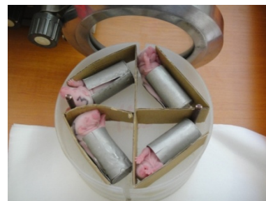
Figure 1 Rats inside the cadmium protection casks and polyethylene holder.
