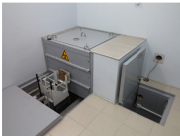
Fig. 1. "Panorama-MEPHI" irradiation chamber and instrumental box
